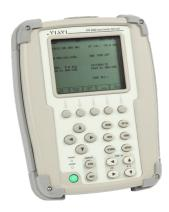
The VIAVI IFR4000 Flight Line Test Set is designed for testing ILS, VOR, Marker Beacon, HF/VHF/UHF Communications (NAV/COMM) Systems, and ELT Short Range Emergency Beacons and 406 MHz COSPAS/SARSAT Long Range Emergency Beacons. The menu-driven functionality and guided test capability make this instrument extremely easy to use.
