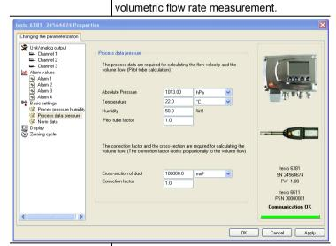
Absolute pressure Absolute pressure existing in the process. The entered absolute pressure value is included in the Pitot tube calculation.
