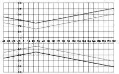
Grey line: System error 6381 + probe, electronics 25 °C/+77 °F
