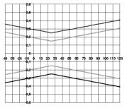
Grey line: System error 6381 + probe, electronics 25 °C/+77 °F
