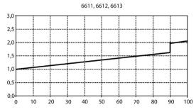
Temperature error as a factor of process temperature and temperature of electronics
