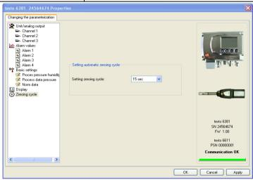
The accuracy specifications are only valid for the zeroing cycle of 15 sec set by the factory.
