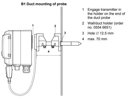
Only atmospheric processes up to approx. 1000 hPa positive pressure. Alternatively, the single-hole duct holder (order no. 0554 1793) can also be used.
