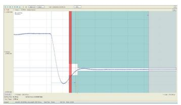
Settling time measurements (Opt. SVT) are easy and automated. The user can select measurement bandwidth, tolerance bands, reference frequency (auto or manual), and establish up to 3 tolerance bands vs. time for Pass/ Fail testing. Settling time may be referenced to external or internal trigger, and from the last settled frequency or phase. In the illustration, frequency settling time for a hopped oscillator is measured from an external trigger point from the device under test.
