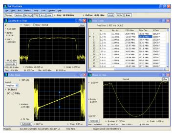
The Advanced Signal Analysis package (Opt. SVP) provides 27 individual measurements to automatically characterize long pulse trains. An 800 MHz wide LFM chirp centered at 18 GHz is seen here with measurements for pulses 7 through 18 (upper right). The shape of the pulse can be seen in the Amplitude vs. Time plot shown in the upper left. Detailed views of pulse #8's frequency deviation and parabolic phase trajectory are shown in the lower two views.
