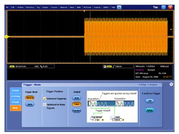
Powerful oscilloscope triggers allow the user to capture only the relevant portion of wideband signals. Pinpoint trigger functions such as combining A and B events with Edge with Holdoff can capture a pulse train during a specific transmitter mode of operation.
