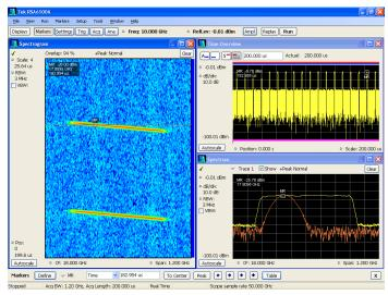
Once captured into memory, SignalVu provides detailed analysis in multiple domains. The spectrogram display (left panel) shows the frequency of an 800 MHz wide LFM pulse changing over time. By selecting the point in time in the spectrogram during the On time of the pulse, the chirp behavior can be seen as it sweeps from low to high (lower right panel).
