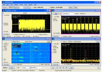
Time-correlated, multidomain view provides a new level of insight into design or operational problems not possible with conventional analysis solutions. Here, the hop patterns of a narrowband signal can be observed using Spectrogram (lower left) and its hop characteristics can be precisely measured with Frequency vs Time display (upper left). The time and frequency responses can be observed in the two right-hand views as the signal hops from one frequency to the next.
