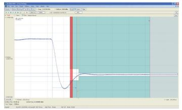
Settling time measurements (Opt. SVT) are easy and automated. The user can select measurement bandwidth, tolerance bands, reference frequency (auto or manual), and establish up to 3 tolerance bands vs. time for Pass/ Fail testing. Settling time may be referenced to external or internal trigger, and from the last settled frequency or phase. In the illustration, frequency settling time for a hopped oscillator is measured from an external trigger point from the device under test.
