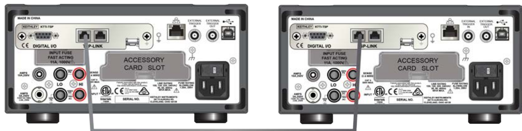
Figure 42: Two DMMs connected with TSP-Link
