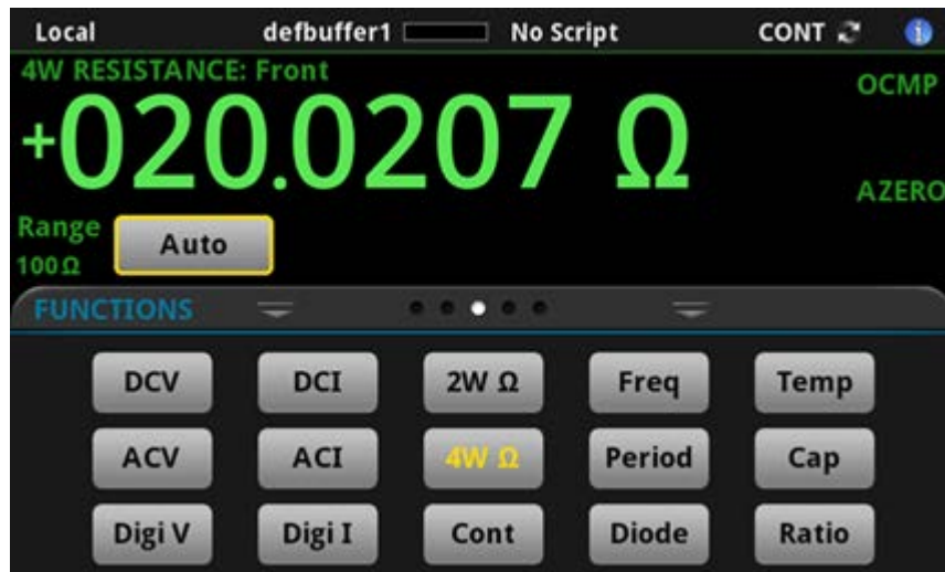
Figure 36: 4-wire resistance test results
