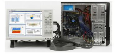
Verification and debug of today's high speed, low voltage DDR Memory interface signals requires probing solutions that can accurately acquire from a wide variety of form factors and provide excellent signal fidelity. Tektronix logic analyzer probes contain a variety of connectivity options that are engineered to ensure that signal acquisition is a true reflection of your design's performance.
