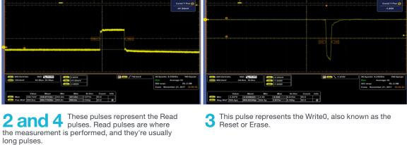
Figure 12: Set, Read, Reset, and Read Cycle Output by the AWG and measured with the scope.
