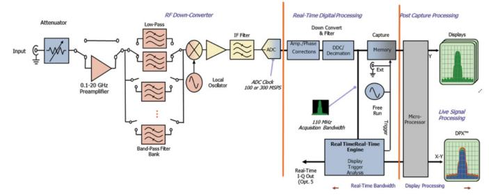
Figure 8. Block diagram of the Tektronix RSA6100 Real-Time Signal Analyzer.
