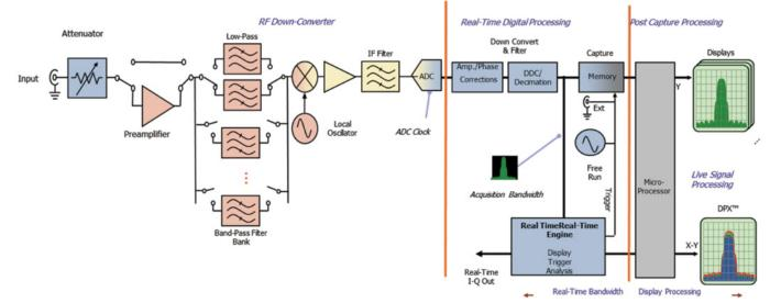
Figure 3. Block diagram of a Real-Time Signal Analyzer (RSA).
