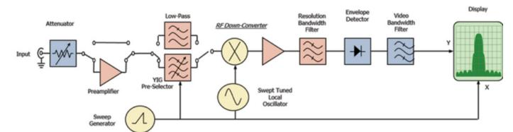
Figure 1. Block diagram of a traditional swept-tuned spectrum analyzer.
