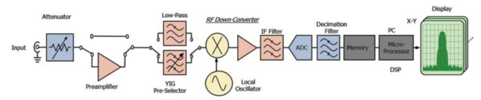
Figure 2. Block diagram of a modern spectrum analyzer with DSP.
