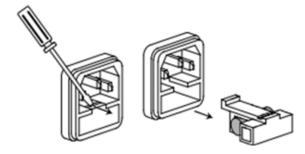
c. Change the fuse based on the machine model. Refer to the table in the below to
