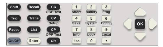
Figure 2 Keypad on the front panel
