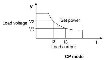
Figure 8 Voltage-current relation under CP mode
