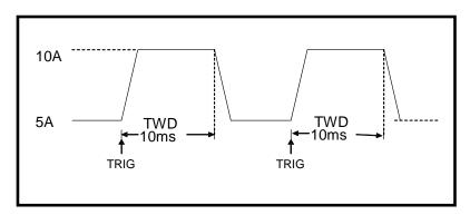
Figure 10 Dynamic test in pulse mode
