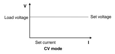
Figure 6 Voltage-current relation under CV mode
