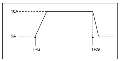
Figure 11 Dynamic test in toggle mode
