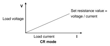
Figure 7 Voltage-current relation under CR mode
