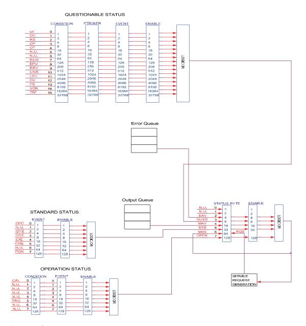
Figure 18 Status register structure
