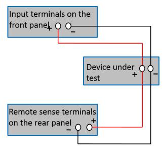
Figure 16 Remote sense connection
