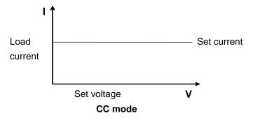
Figure 5 Voltage-current relation under CC Mode
