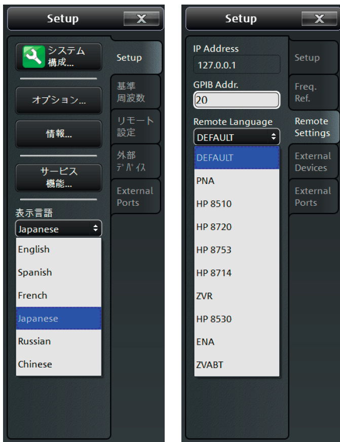
Soft panel menus for selecting language (left) and remote control command set (right).
