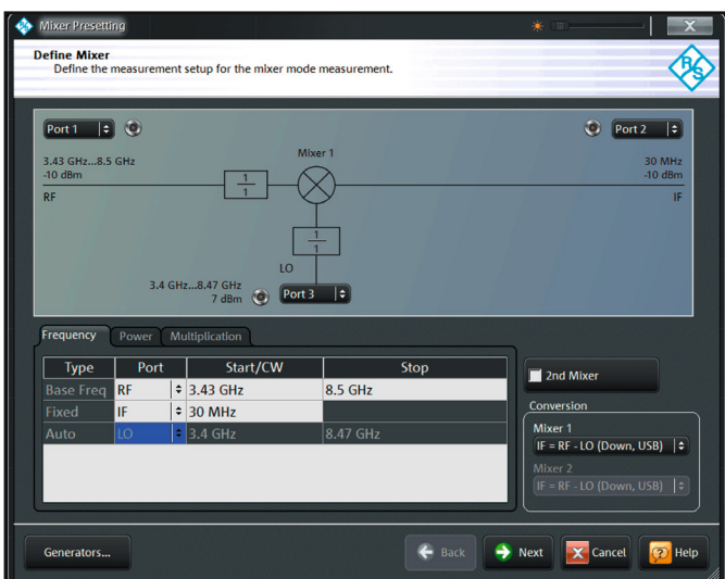
Wizard for configuring mixer measurements.
