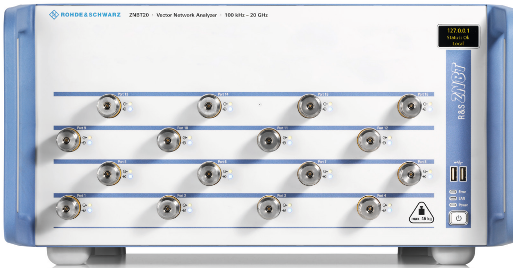
The R&S®ZNB20 with 16 ports.
