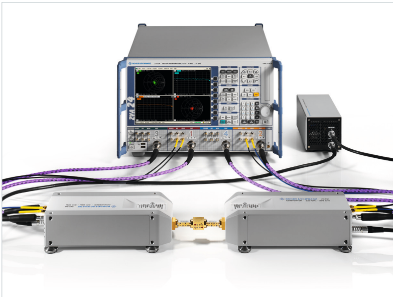
Setup for a two-port measurement in WM-864 band with an R&S®ZVA24 vector network analyzer.
