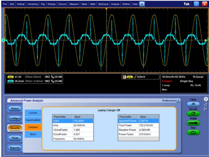
Figure 12. Power Quality Measurements on a PC power adapter after the laptop battery is charged, with the laptop turned off.
