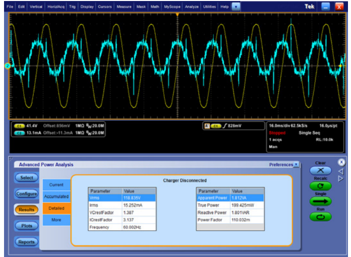
Figure 13. Power Quality Measurements on an unloaded laptop PC power adapter.
