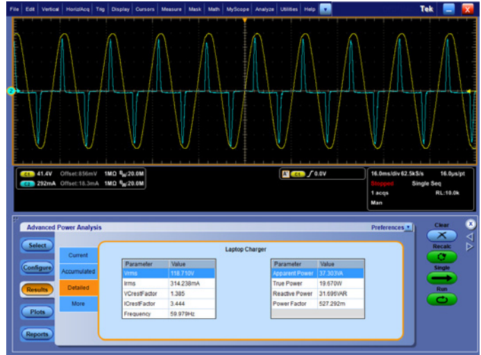
Figure 11. Power Quality Measurements on a PC power adapter after the laptop battery is charged while the laptop is running.
