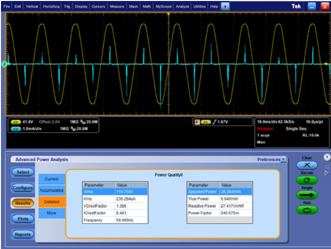
Figure 15. Power Quality Measurements on a cell phone charger after the phone is charged.
