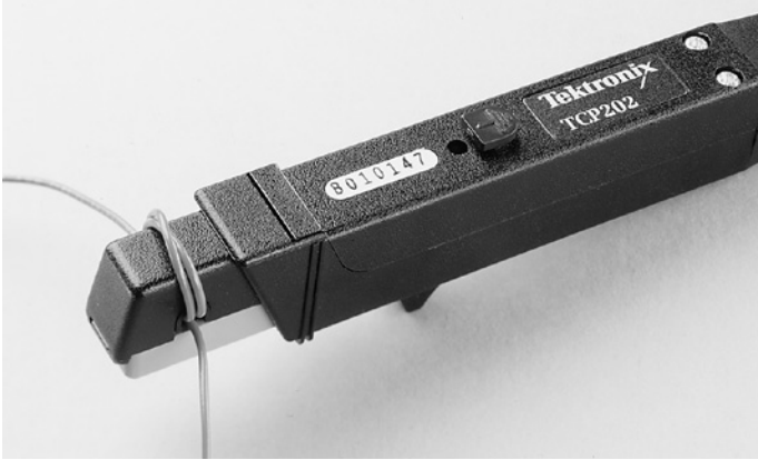
Figure 5. Increasing current sensitivity by wrapping N turns of the conductor around the current probe.
