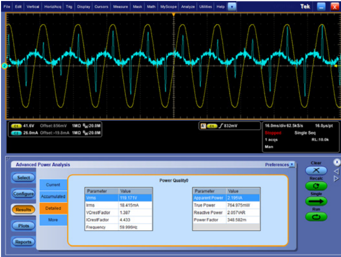
Figure 10. Power Quality Measurements on an LCD monitor in standby power mode.
