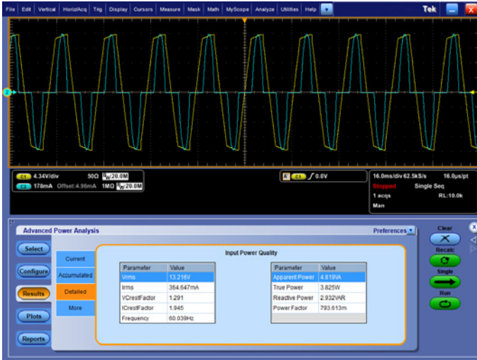
Figure 8. Voltage, Current, Power, and Energy Readouts.
