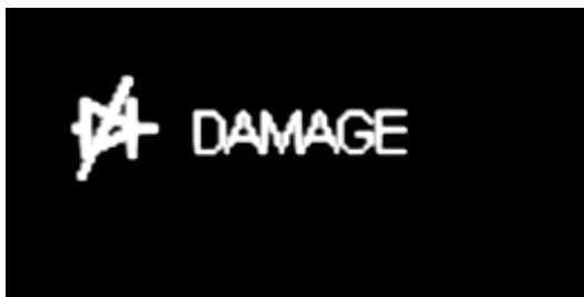
Figure 3-14: Display of Diode Measurement (Damaged Diode)
