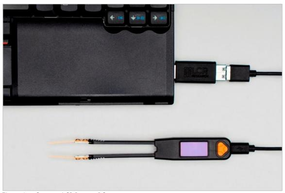
Figure 3-1: Connect LCR Pro1 to PC
