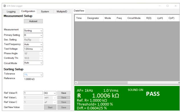
Figure 5-2: Sorting Screen with Passed Result
