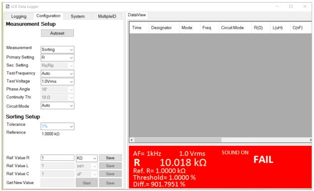
Figure 5-3: Sorting Screen with Failed Result
