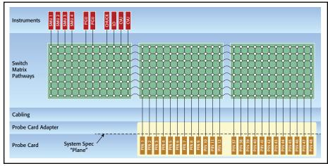
Every \$530 system is made up of five layers: instruments, switch pathways, cable interface, probe card adapter, and probe card.
