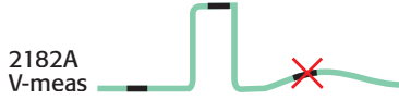
Figure 2. Heat generated by the pulse in the DUT or contacts may corrupt the third measured point, so it may be discarded.
