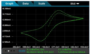
Figure 3. Voltammogram generated with Model 2450 SourceMeter SMU instrument
