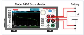
Figure 12. Results of discharging battery shown on graphical display of Model 2460 SourceMeter SMU instrument
