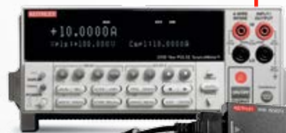
First one-kilowatt pulsed SMU instrument (Model 2430)
