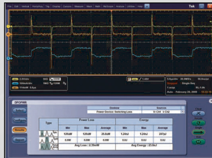
DPOPWR switching loss measurements.
