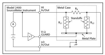
Figure 5. Model 2400's Built-In Guard.
