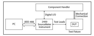
Figure 2. 2400-Based Resistor Production Test System..
