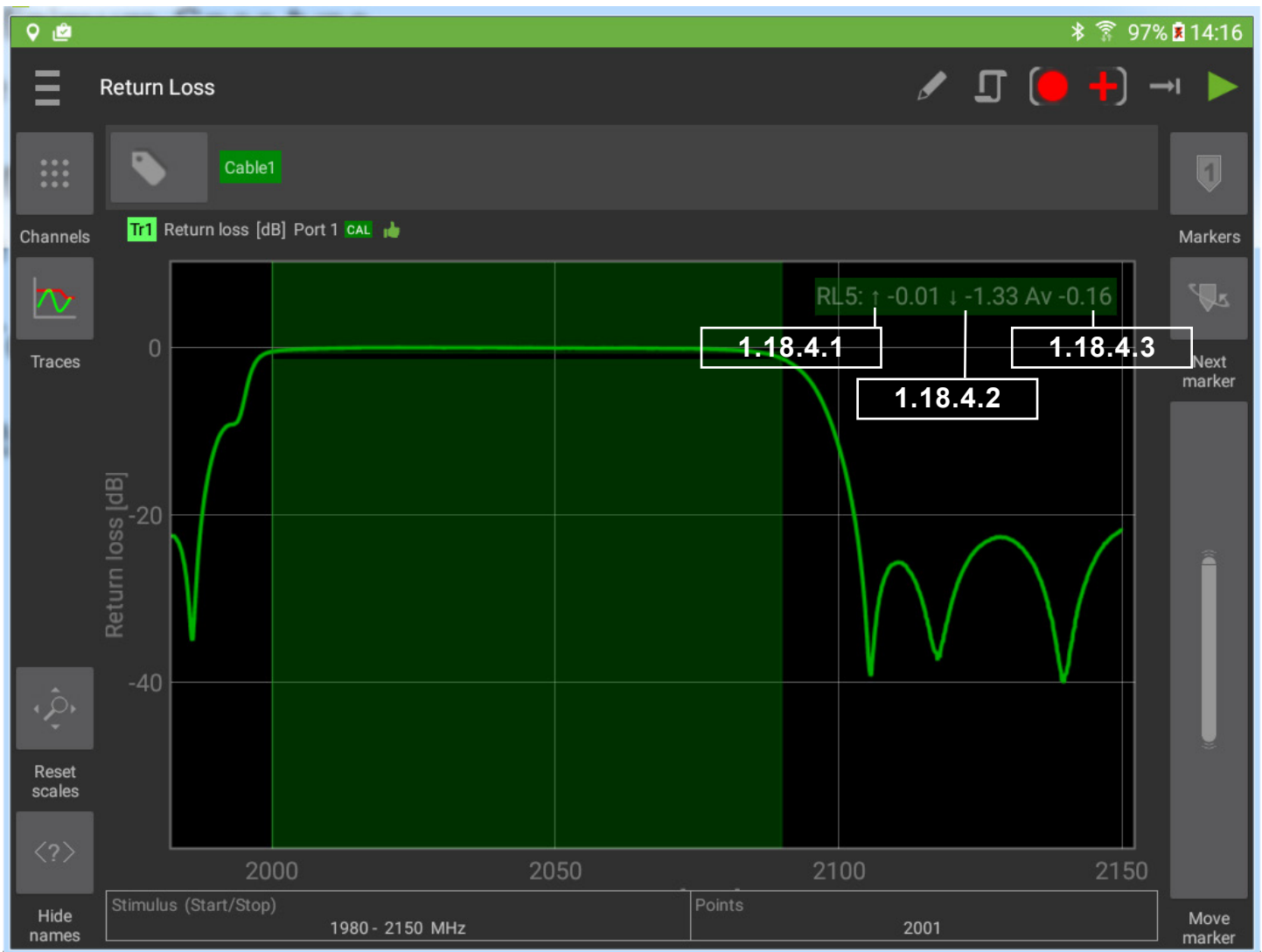
Figure 20 Ripple Limit on a Trace
