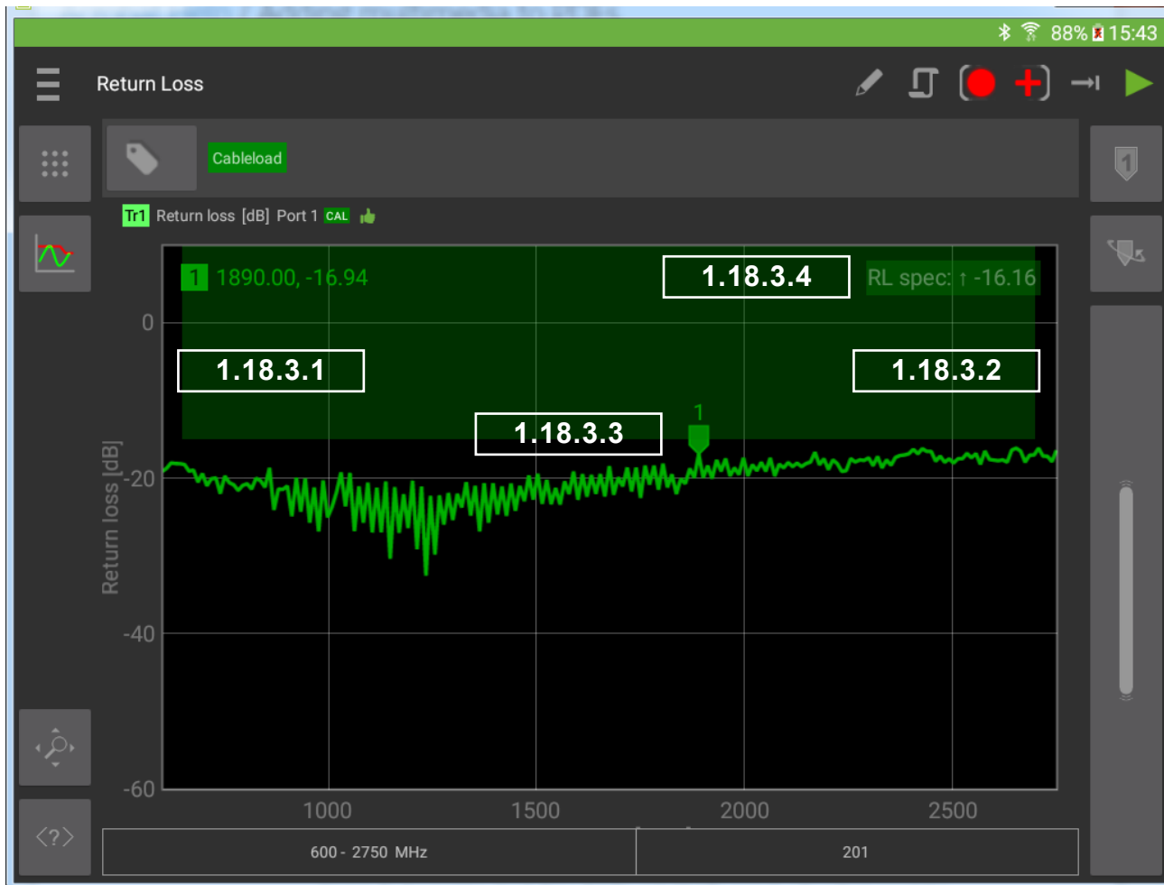
Figure 19 Max Limit Drawn on a Return Loss Trace
