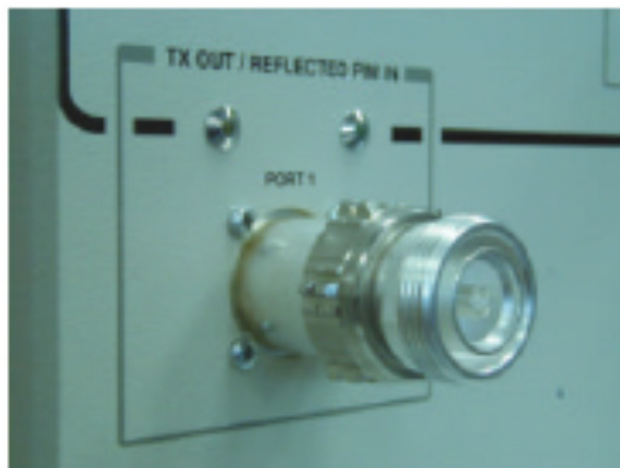
Figure 1. Front panel 7-16 connector with connector saver
