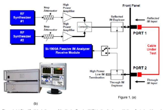
Figure 1. (a) Simplified block diagram of the Kaelus Passive IM Distortion Analyzer with the reflected and through IM responses of interest. (b) Photo showing the analyzer used to measure the cable assembly.
