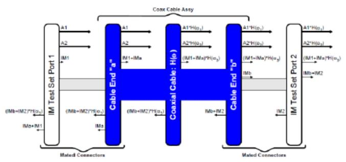
Figure 2. Model used to formulate the reflected and through IM response characteristics of a cable assembly.
