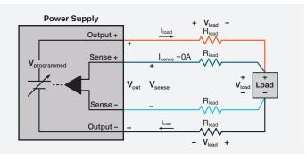
Ensure that the Programmed Voltage is Accurately Delivered to the Load
