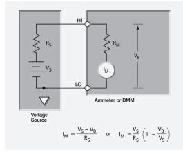
Effects of Voltage Burden on Current Measurement Accuracy
