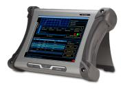
The VIAVI ALT-8015 is the world's first and only RF-based portable radio altimeter flight line test set. The ALT-8015, designed for military applications, tests from the TX/RX antennas to the indicator in the cockpit, allowing the operator to replicate inflight conditions and isolate a bad component of the installed system.
