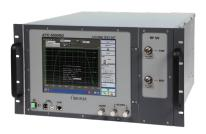
The VIAVI ATC-5000NG is an RF signal generator/ receiver for testing Mode 3/A, C and S transponders. The ATC-5000NG was designed with modern software defined radio technology and is the replacement product for the commercial functionality of the SDX-2000, ATC-1400A and S-1403DL. The ATC-5000NG is capable of performing most MOPS tests for DO-181E, DO-260, DO-260A, DO-260B, and DO-282B and is the ideal test equipment for engineering development, certification, manufacturing and service.
