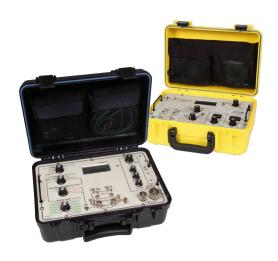
VIAVI fuel quantity test sets will accurately test or troubleshoot any AC or DC capacitive fuel, water, LOX, Engine Oil or other AC or DC system when used with VIAVI aircraft specific interface cables/units.
