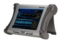
The VIAVI ALT-8000 is the world's first and only RF-based portable radio altimeter flight line test set. The ALT-8000 tests from the TX/RX antennas to the indicator in the cockpit, allowing the operator to replicate in-flight conditions and isolate a bad component of the installed system.
