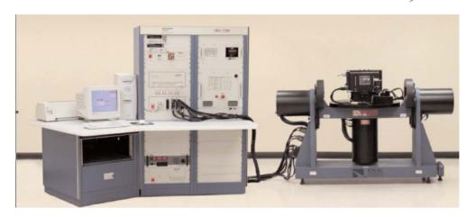
The IRS1200 is an inertial reference test system used to test Honeywell Air Data Inertial Reference Units (ADIRU) and Inertial Reference Units (IRU) of air transport, commuter and business aircraft, as well as cockpit control panels and system display units.
