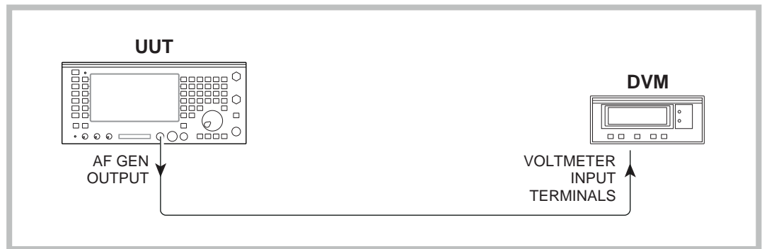
Fig. 5-10 Audio generator level accuracy checks
