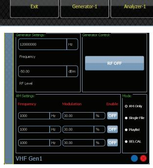
**VHF Gen** - Provides control of modulation frequency, modulation depth (up to 3 sources), SELCAL tones, frequency and tone sequences.
