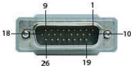
Fig. A-6 AUX Connector Pin-Out Diagram
