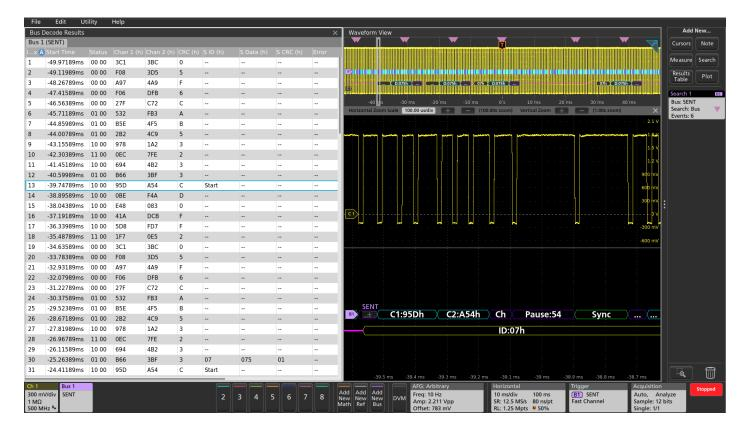
For firmware engineers, the Results Table format may be more useful. This time-stamped display of bus activity can be easily compared to software listings, and allows easy calculation of the execution speed.
