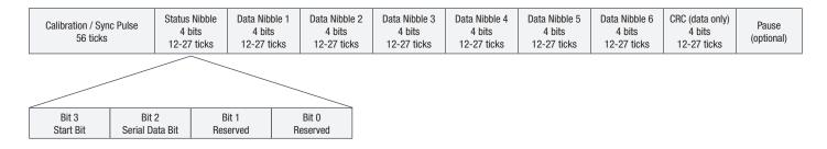
The physical layer of the SENT interface consists of a signal line, a +5V supply voltage line, and a ground. The signal line logic levels are low < 0.5V and high > 4.1V.
