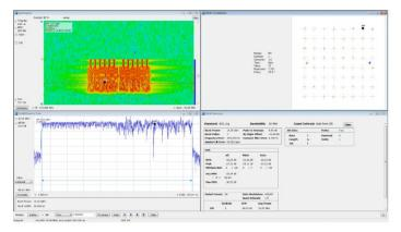
SignalVu-PC Option MAP enables interference hunting and signal strength analysis. Locate interference with azimuth direction function. It lets you draw a line or an arrow on a mapped measurement to indicate the direction your antenna was pointing when you take a measurement. You can also create and display measurement labels.
