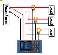
Pulse Input The pulse input function can be used to record power data and production volume counts simultaneously. The power data and pulse volume (production volume) information are useful for unit cost production management.
