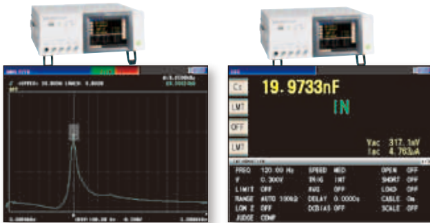
Frequency sweep measurement Z peak comparator screen
