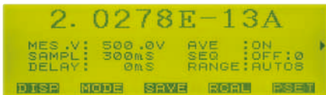
Data display with 0.1 fA resolution (10 pA range).
