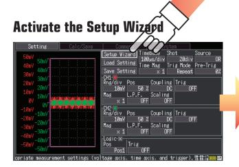
When powered on, the Settings screen appears along with the waveform monitor, and the new Setup Wizard blinks. By activating the Setup Wizard, you can easily navigate by following the simple instructions. Soon you will be operating the device like a seasoned professional.
